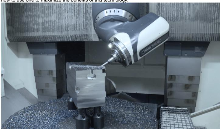
The most common type of 5 axis machining involves two rotational axes. These axes can be independently moved and are often complex geometry. You can also cut multiple parts at once. This enables you to get larger, more accurate parts faster. The machine can also be programmed to make multiple parts per cycle. Depending on your needs, a 5-axis machine will allow you to produce more than one part in a single cycle.
