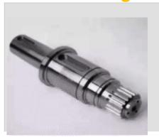
An advanced CNC turning-milling compound lathe processes the stainless steel motor spindle, and all processing procedures can be completed in one clamping. The size tolerance range is ±0.02mm, and the surface is passivated and cleaned.
