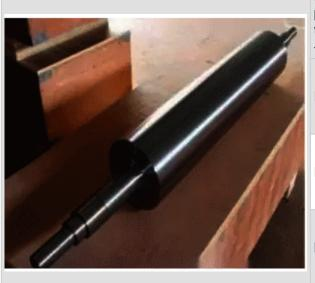
Large-scale roller, the blank is made by the hot drying sleeve process, after welding, it is turned into a whole by a CNC lathe, the surface is polished, and the tolerance of the bearing gear is +0.005
